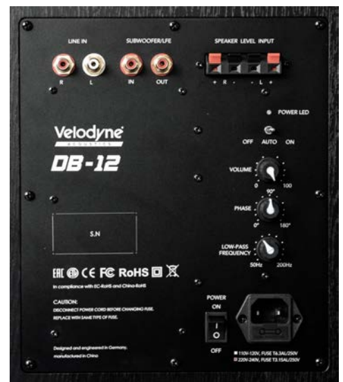
Back Panel with Audio input and Volume/Phase/ Low Pass Filter control
