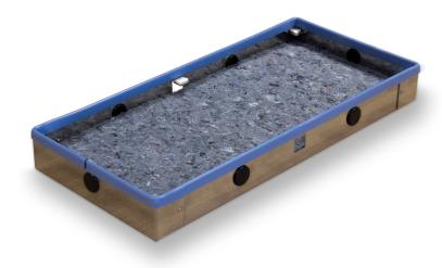
The front of the alignment trim sits such that it represents the level of the front of the speaker once installed, therefore it can be used to accurately position the backbox and achieve correct speaker alignment.
