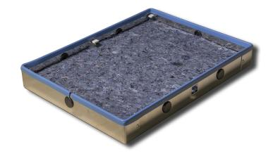
Alignment trim should be left in place whilst render is applied to the wall, only to be removed immediately prior to speaker installation. Recycled denim insulation should be removed temporarily during render application and re-installed immediately prior to speaker installation. All voids surrounding the BackboxSW should be filled with expanding foam.
