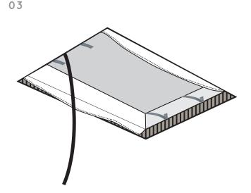
Position firehood up into ceiling void. Position centrally to aperture. The two large end flaps should be folded outward. The side flaps should be either folded inward and pinned to the back of the plasterboard, or positioned against the cut edge of the plasterboard and pinned into place
