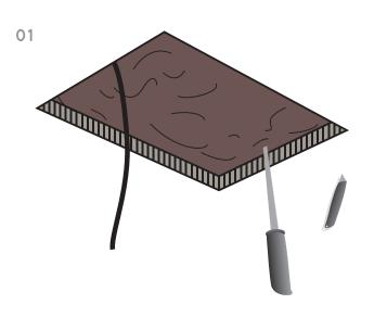
Cut hole in plasterboard as per speaker/backbox instructions. It may be necessary to increase the hole width by up to 10mm to allow the firehood side flaps to be positioned between the speaker's edges and the plasterboard. If there is enough space between the ceiling joists the firehood's side flaps can be folded inward and positioned against the back of the plasterboard.
